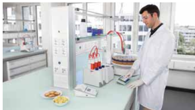
Figure 2: METTLER TOLEDO's Titration Excellence line allows fully automated sodium determination. Automating the process with the InMotion™ Sample Changer increases efficiency and provides a much higher throughput
